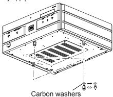
The feet can also be attached to the back-side holes. If the front side of the device is not stable, attach the feet to the back-side holes.
